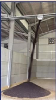
storage silo and a 29tph, PLC panel operated, continuous mixed flow drier, all of which was supplied and manufactured by Perry of Oakley Ltd. to maximise the efficiency of the store. With the new throughput capacity of 2500 tonnes per year at Catton Farms, the standard Perry equipment copes with ease. The machines selected were the Perry standard Agricultural range with a 3mm thick galvanised steel base and 2mm thick galvanised steel sides to ensure maximum machine life.
