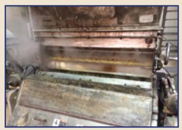
water dosage. It is a stainless steel measuring channel with online temperature, moisture & hectolitre weight measurements.
