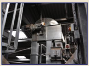
From the drier, the dried grain is then passed through a second aspirator pre-cleaner, then up another belt & bucket elevator and then delivered to stores via a belt conveyor which has been installed with a motorised tripper, allowing John & Allan Marshall to make the most of the storage space available in their new buildings and existing stores.
