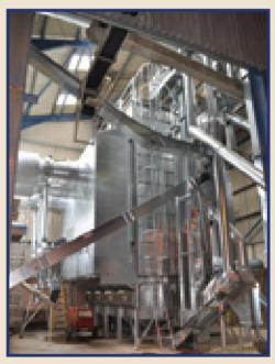
The new installation at Revesby Estate is an intricate network of conveyors, elevators, aspirator cleaners, cyclones, ducting and a drier.
