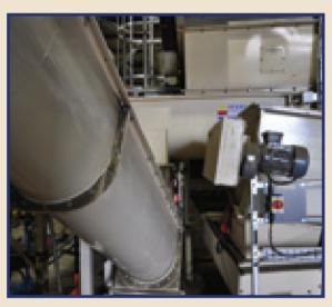
The screw conveyor lengths range from 3m to 8.5m, going from horizontal up to a 25 degree incline. They are durable and adaptable, meaning they are handling the different inclines easily and efficiently. From the point of order, the machines were despatched in just 5 weeks; Perry of Oakley Ltd. had met the targets of the tight deadlines within the time specified.
