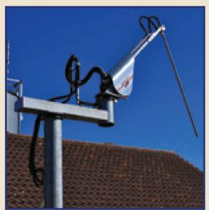
All the electronic components and wiring are enclosed neatly on the sampler pillar. With the limp home mode available, the sampler can operate up/down and swivel drives even if the VFD fails, meaning no down time.
