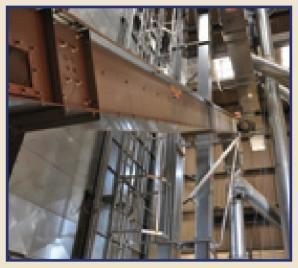
throughput capacities of up to 49tph and has a holding capacity of 51 tonnes. The drier has been fitted with Perry of Oakley Ltd.'s revolutionary CentriKleens, which reduce the amount of dust & chaff exiting the drier by up to 95% (independently verified), helping to keep plant yards and roofs clean. CentriKleens can be retrofitted to any drier with axial fans.
