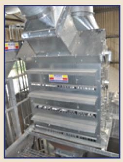
There is one uprated and refurbished existing intake and seven new chain & flight conveyors, one of which is a flow and return conveyor and five are curved combination conveyors. All of the conveyors are capable of achieving 100tph throughput capacity and range in lengths from 9.1m to 26.5m.
