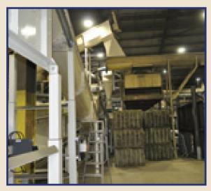
A by-product of exchanging the belt & bucket elevators and conveyors with the screw conveyors has been the reduction of dust in the atmosphere. It is now an almost dust free environment to work in and again helps reduce the risk of fire.
