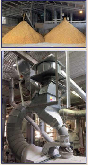
Once the corn has been flaked, the flakes are then discharged directly into a Perry Belt Drier, which takes the moisture content of the flakes from 23% down to 11% by drying and cooling the flakes, which gives the flakes a much longer storage life. The customer installed a 10tph belt drier, but currently only requires it to output approximately 8tph.
