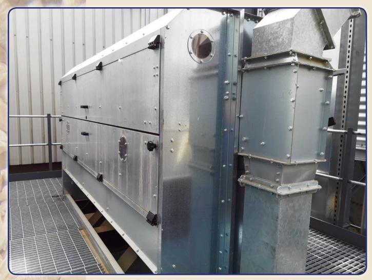
The product enters by gravity into a cylindrical rotating drum with changeable perforated screens. The good product passes through pre-set holes, while the rough impurities come out at the end of the drum. The choice of screen perforation size depends on the product, the moisture content and the type of reject to separate.
