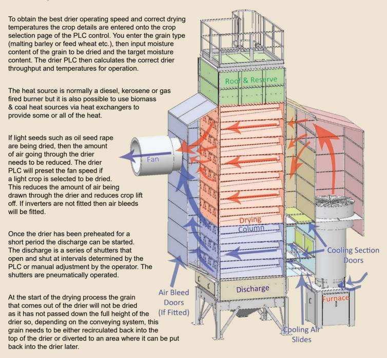
Whilst the drier is running the operator will take periodic moisture samples of grain entering and leaving the drier. When the desired exit moisture content is reached the conveying system is changed so that the dry grain is sent to store and not recirculated.
